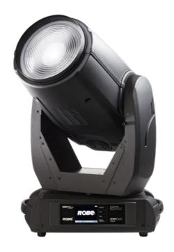
Mechanical features include a newly designed linear motorized zoom of 5.5° - 60° and a diffusion filter for extension of the zoom up to 75°. The fixture uses a internal Barndoor module for creating different shapes. The module consists of four individually controllable blades and is rotatable by plus or minus 90 degrees.
